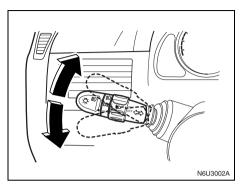
To signal a turn, move the lever all the way up or down. When the turn is finished, the lever will return automatically.
